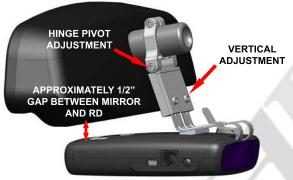
3 - Install the RD onto the mount. Make the necessary adjustments as shown above. Using the vertical adjustment, we recommend you adjust the RD so there is approximately 1/2" gap between the bottom of the mirror and the top of the RD. After all adjustments are made, be sure to check that the hinge pivot and vertical adjustment screws are tight. The screw on the very top of the mount should be tightened last.
